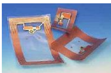
Fig. 1. Sticker RFID tags used by post parcels
